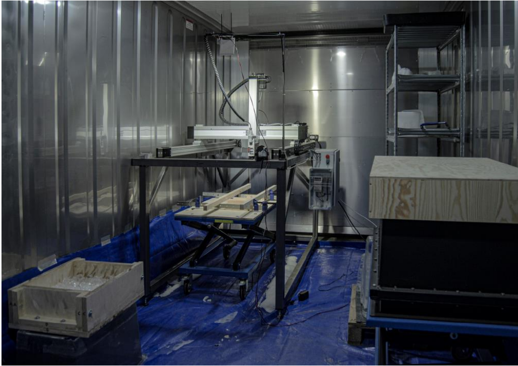
Fig. 3 – CNC machine and ice stock generator installed in the refrigerated container
