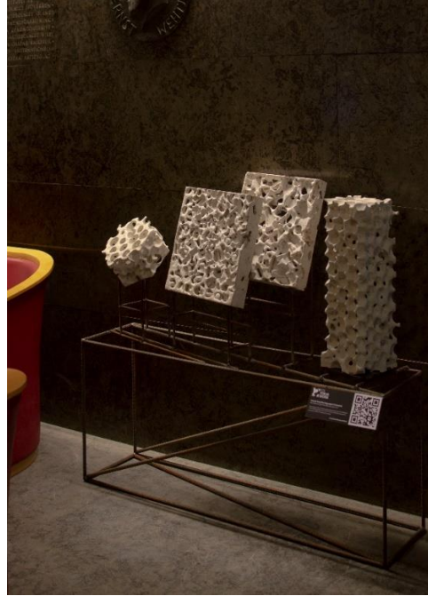
Prototypes 1 and 2 - (Left) Light-Weight Rain-Screen Facade Element (Right) Packed-Fused Ice Aggregate Formwork
